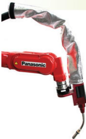
Wire Wizard supplies a range of cable sleeves made out of Kevlar with an Aluminized coating. These sleeves protect your costly cable assembly for wear and welding spatter. The sleeve is made with a heavy duty zipper and a Velcro enclosure to seal it tightly.
