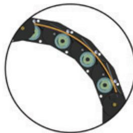
Internal view showing the path of the wire along rollers.
